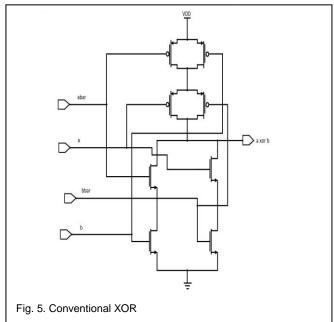
PTL implementation of XOR gate results in use of less number of transistors, in turn results in less energy consumption for arithmetic functions which contains XOR gates.
