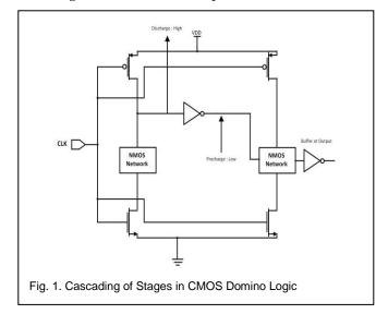
When the clock is low, dynamic node is pre charged to high and the output of the first buffer will become low. nMOS present in the next logic block will be in OFF condition. When the clock goes to HIGH, dynamic node is conditionally discharged and the output at the buffer will simultaneously go to HIGH International Journal of Scientific & Engineering Research Volume 4, Issue 8, August-2013 ISSN 2229-5518
