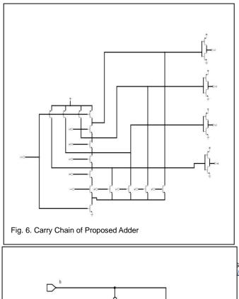
The Fig. 5, Fig. 6, circuit diagram of the Manchester carry Chain and XOR of the proposed area efficient adder. Here it uses only 22 transistors for implementing Manchester carry chain and 6 transistors for XOR implementation. Thus it shows a reduction of 25% in transistor count compared to the Conventional Manchester adder. The Block representation of the proposed 32 bit adder was shown in Fig.8.
